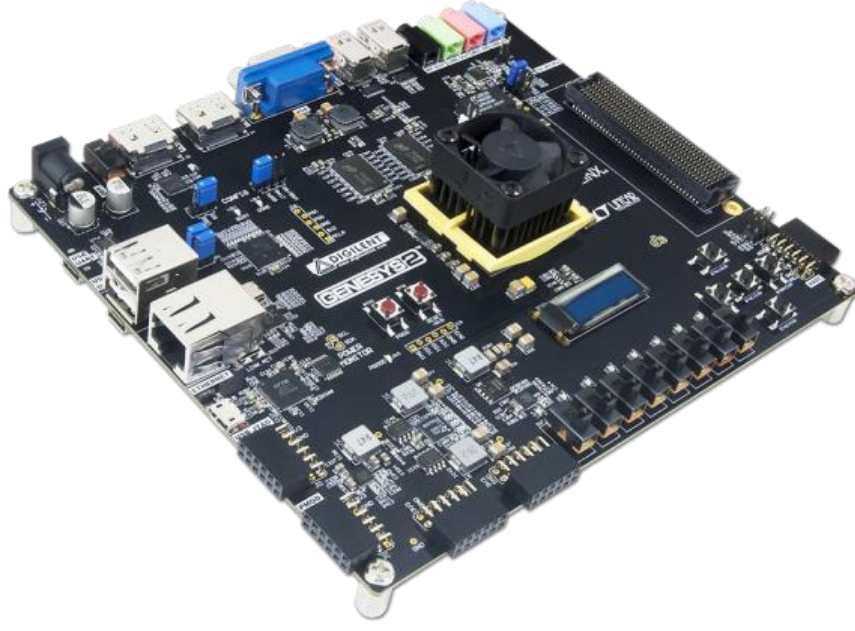
Görsel 2. Xilinx Kintex-7™ FPGA (XC7K325T-2FFG900C) bordu [46]
